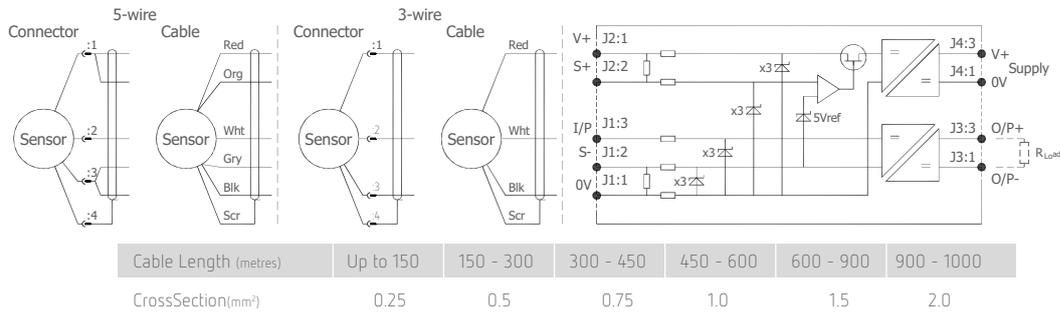
The table above shows recommended conductor sizes with respect to cable length for both three and five wire connections, based on copper conductors. Three wire connections will introduce a gain reduction of 5% and a  $\pm 1\%$  temperature dependence of gain over the range  $-40^{\circ}\text{C}$  to  $+80^{\circ}\text{C}$  for the cable temperature. (i.e. about  $-150 \text{ ppm}/^{\circ}\text{C}$  for the maximum lengths shown and less pro rata for shorter lengths.)
