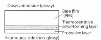
This is the non-glossy surface that comes into direct contact with the heat source. The glossy side of the sheet is used to analyze the color patterns that represent heat distribution.
