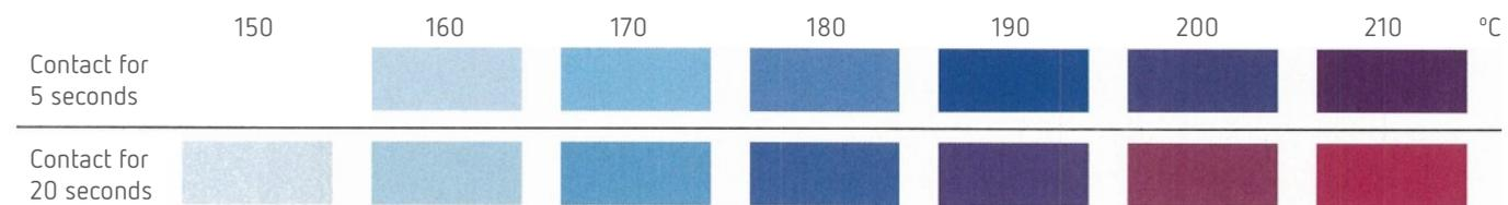
Note: The above chart is a sample based on the results of a test performed at Fujifilm. Before using Thermoscale, create a similar chart that is based on the actual measurement conditions
