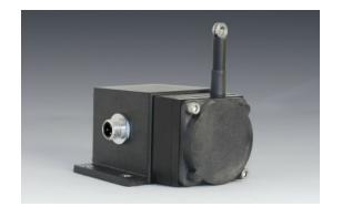
The PT1DC can operate from an unregulated 14.5 to 40 VDC power supply while providing an output signal that is proportional to the linear movement of it's measuring cable. The PT1DC has a maximum measurement range up to 50" and has 4 output signal options to choose from: 0...10, 0...5, -10...+10 and -5...+5 Vdc.
