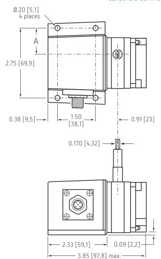
\* tolerance = +.005 -.001[+.13 -.03]\*\* tolerance = +.005 -.005[+.13 -.13]
