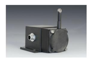
The PT1DN communicates to your PLC over DeviceNET® and provides a precision position feedback signal for full-scale measurement ranges from 2 to 50 inches. Because the PT1DN uses a potentiometer as it's sensing element, the position signal is "absolute" and does not have to be reset to a "home" position upon startup.
