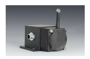
The PT1MA adds 4...20 mA position feedback signal to our compact line of cable-extension transducers. The PT1MA is available with full stroke ranges from as little as 2 inches on up to 50 inches with adjustable zero and span settings to precisely match the full scale output to your exact measurement range. The PT1MA offers several options including forward and re- verse 0...20 and 4...20 mA output signals, alternate measuring cable exits and a couple different electrical connection options.
