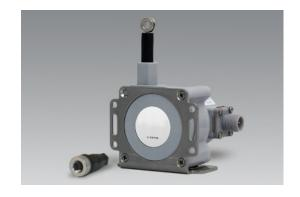
This compact stringpot provides the ultimate in ease-of-use and flexibility. This sensor fits in small spaces, doesn't need perfect alignment, mounts in just about any direction imag- inable and has a unique circuit that lets the user choose 4-20mA or 0-10Vdc output on the fly.
