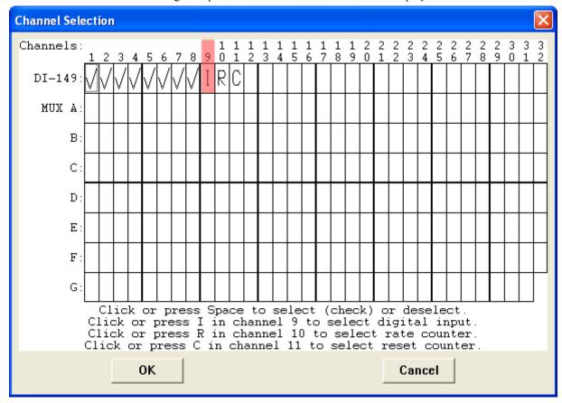
Channel 9 records and displays all the digital inputs, even the state of the Rate and Count inputs if those channels are enabled. With Channel 9 selected in the display window click **Scaling** > **Digital Plot** to show a digital display and make the data more meaningful on screen.
