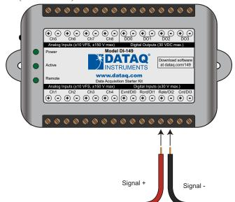
Connect any TTL pulse stream (30 VDC max) to the Rate/DI2 channel on the DI-149.
