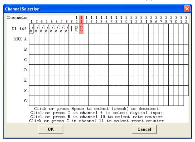
The counter channel accumulates counts over time whether recording or in standby mode as soon as the Counter channel is enabled. The *accumulated* values will be recorded to your data file unless you reset the counts to zero. The maximum count value is 16383 before the counter resets to zero automatically.
