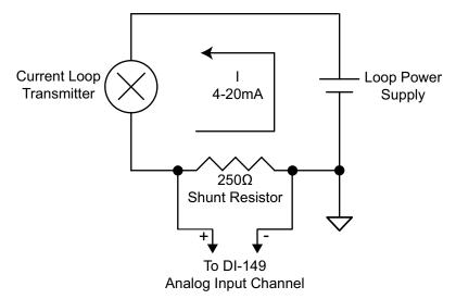
Set the engineering units as desired and define low/high calibration values in WINDAQ as 1V = 4mA for the low value and 5V = 20mA for the high value. For example, when using WINDAQ Acquisition software, in the Channel 1 Low Calibration dialog box:
