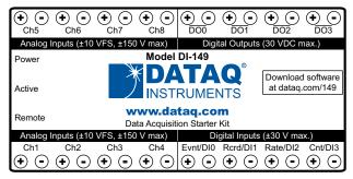
Analog Inputs Ch#: Analog channels 1-8 (±10VFS, ±150V transient max.)
