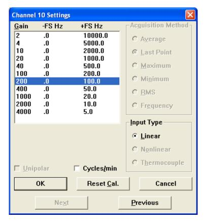
Check the "Cycles/min" box to display and select frequencies reported in cycles per minute instead of cycles per second (the measurement interval remains the same). Tachometer measurements in units of RPM (revolutions per minute) is just one example that benefits from selecting this option. For example, if the 100 Hz range setting is selected and "Cycles/min" is checked, the full scale range is actually 6000 cycles per minute.
