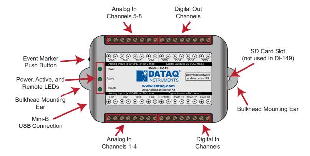
**Please note:** The SD card slot is not used in the DI-149. Allowing foreign materials to enter the device through the SD card slot may result in damage to the instrument.
