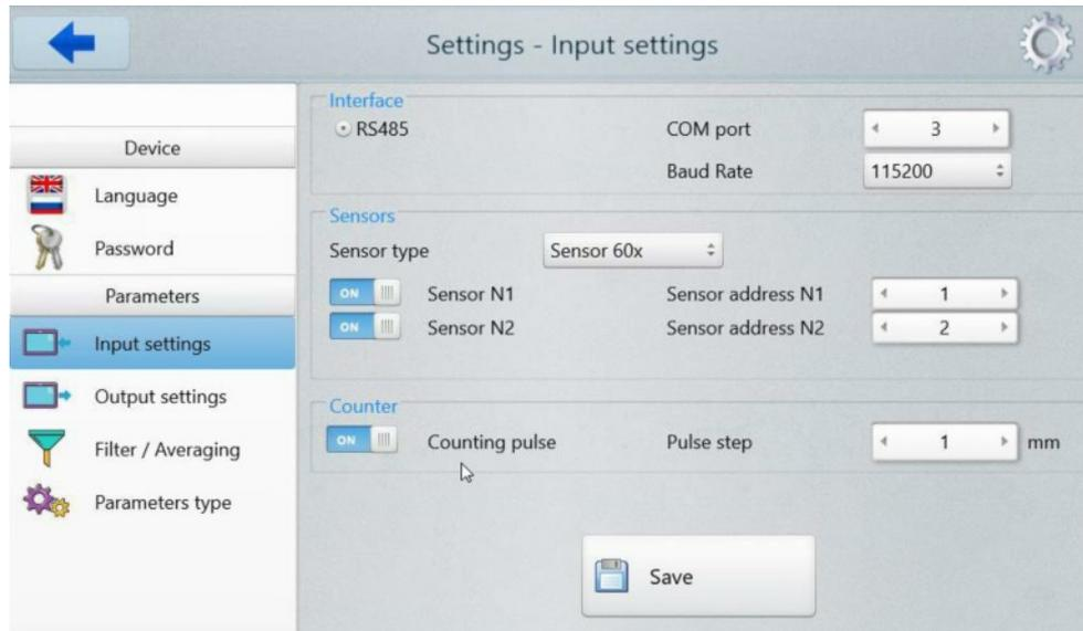
The **Input settings** tab for the two points measurement system:
