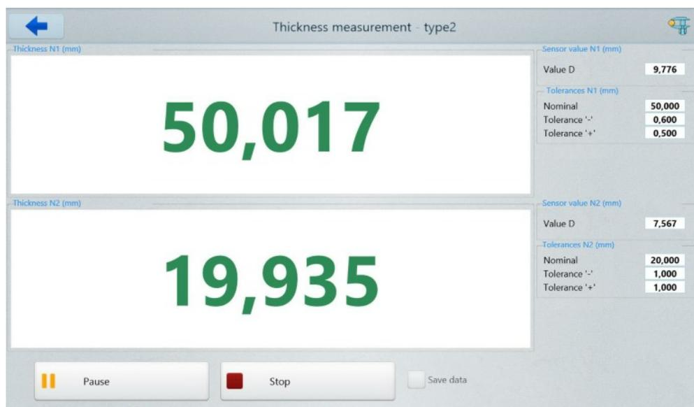
If needed, you can tap the **Stop** button to stop the measurement process, or tap **Pause** to pause the measurement process.
