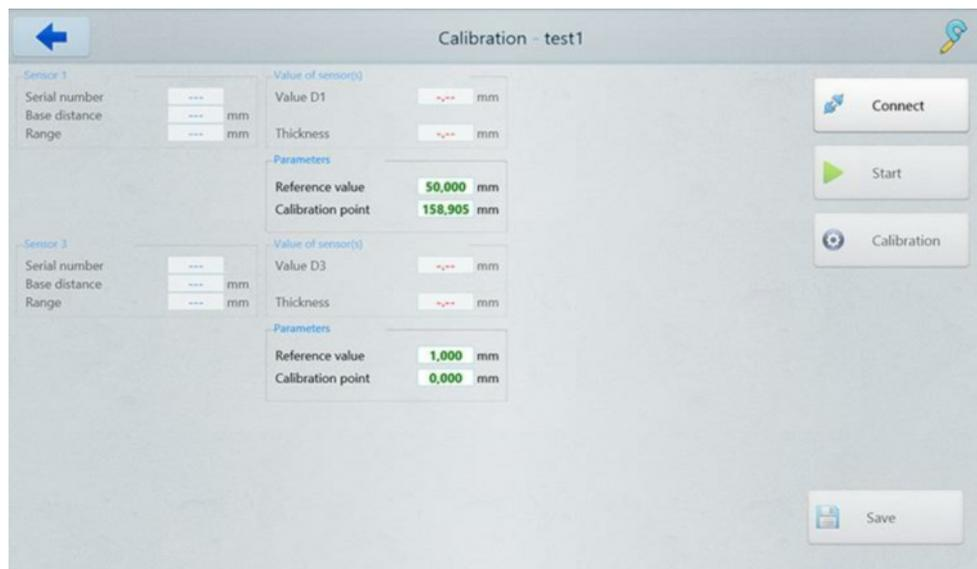
• Tap the **Connect** button in order to connect to the sensors.
