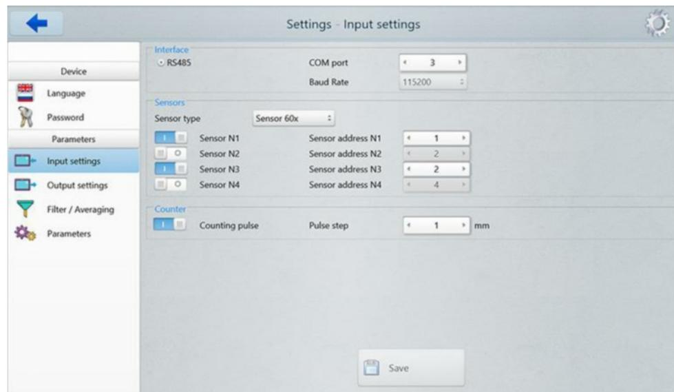
In the Interface settings area, the user can specify the COM port number and the baud rate.
