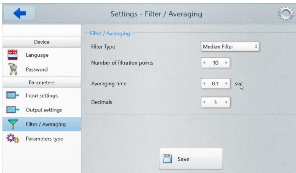
Filtering is intended to lower the noise of the measurement signal which results in a better resolution. The description of parameters is given in the table below.
